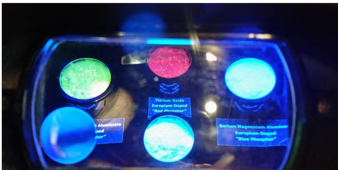
Figure 9. The view when looking into the phosphor viewing box. This photo shows the rare earth-doped phosphors illuminated with longwave UV light. Note that the obstruction on the bottom left of the image is from a built-in magnifying lens and is not present when actually viewing in-person.
