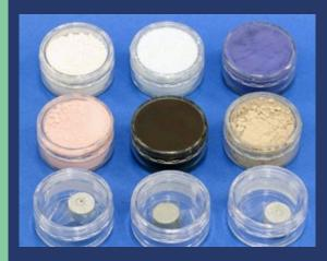
These rare earth elements and cobalt products were recovered from waste magnets, including those contained in electronic waste, via the acid-free dissolution process. Permanent magnets were remade with the recovered rare earth products.
