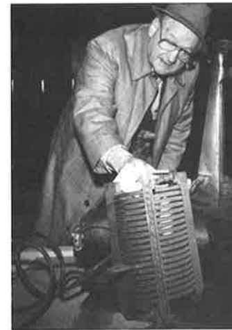
Wilhem inspects an induction coil used during the process to make pure uranium ingots.
