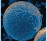
Ames Laboratory's specialized **gas atomization** method efficiently produces customizable metal powders for advanced manufacturing. The process has resulted in numerous patents and led to a spin-off company, Iowa Powder Atomization Technologies, that was later acquired by the Fortune 500 company Praxair as part of a major commercialization effort.
