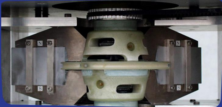
A prototype magnetic refrigerator.
